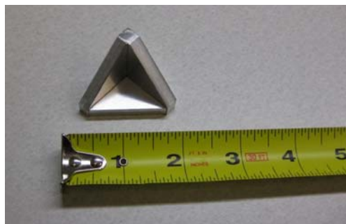
Figure 10. Small (1.5-in.) Corner Reflector Used to Mark 100-ft Increments on the Long Axis of the Test Rectangle
