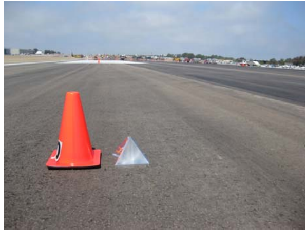
Figure 8. Cones and Large Corner Reflector Marking Front-Left Corner of the Test Rectangle
